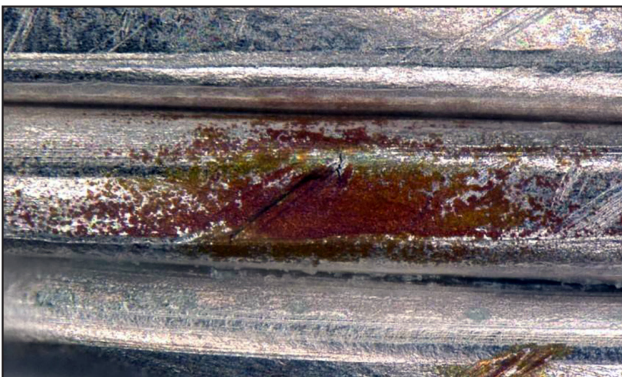
Figure 1-2 - Red Plague (Cuprous Oxide Corrosion)
