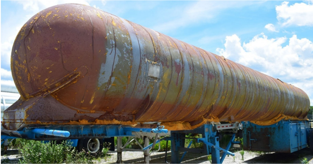
Figure 1—Example of trailer with insulation removed
